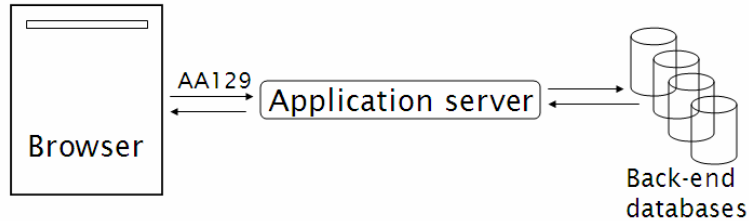
► Figure 19.1 A dynamically generated web page. The browser sends a request for flight information on flight AA129 to the web application, that fetches the information from back-end databases then creates a dynamic web page that it returns to the browser.
